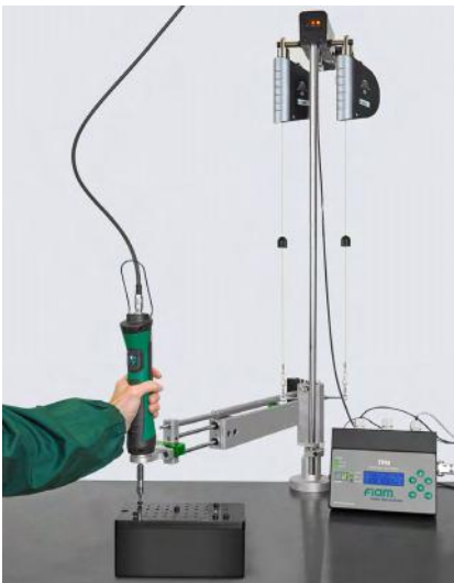
Cartesian arm with a position monitoring device.
