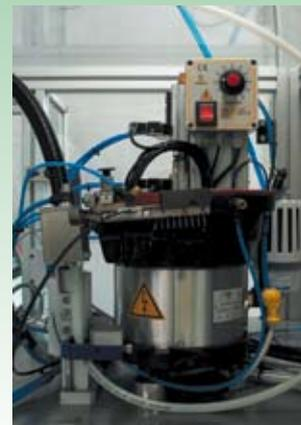
Detail of screw feeding system with optical fibre and amplifier
