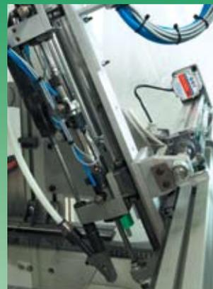
Detail of electric axis on three positions
