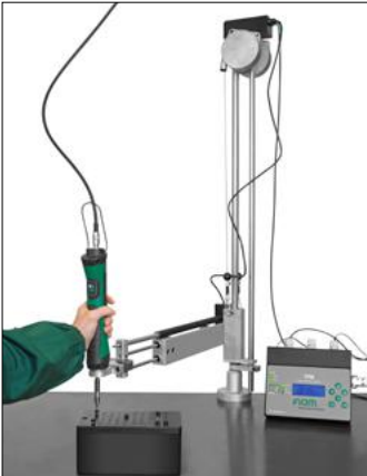
Cartesian Arm with a position monitoring device
