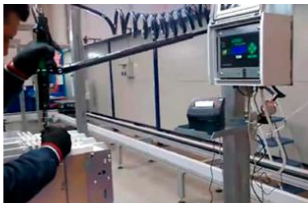
Process under control and print of tightening results
