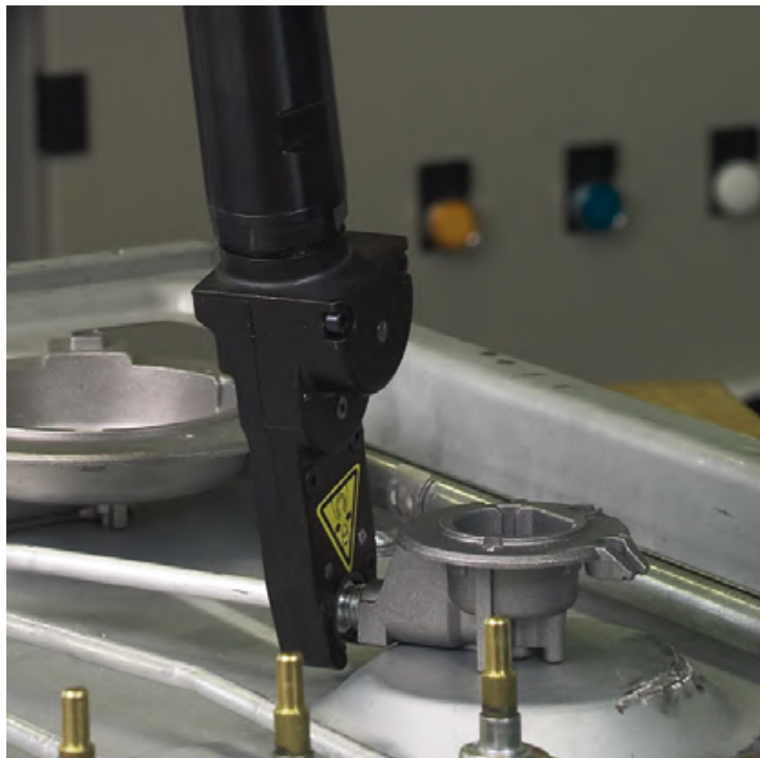
Radial opening ideal to reach the nut.
